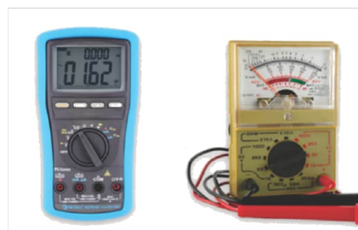
Fig. 16.3: Comparison of digital and analog ammeters
